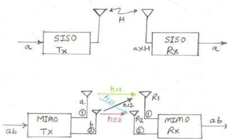
Fig 2. Operational Difference between SISO & MIMO
