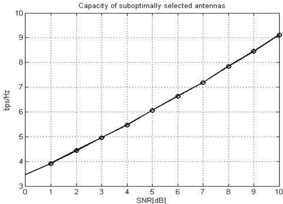
Fig 4. Channel Capacity for MIMO
