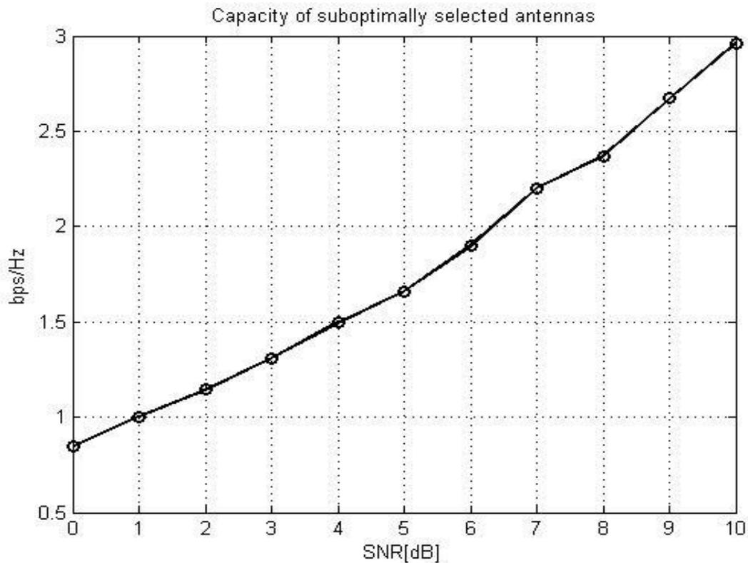
Fig 3. Channel Capacity for SISO
