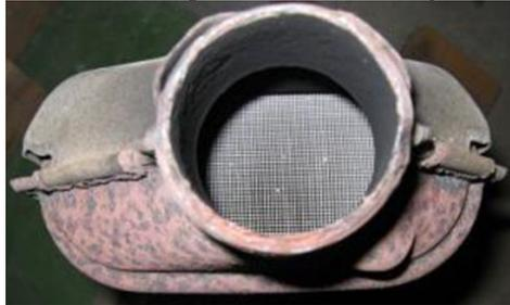
Fig. 4: Ceramic core converter [3].
