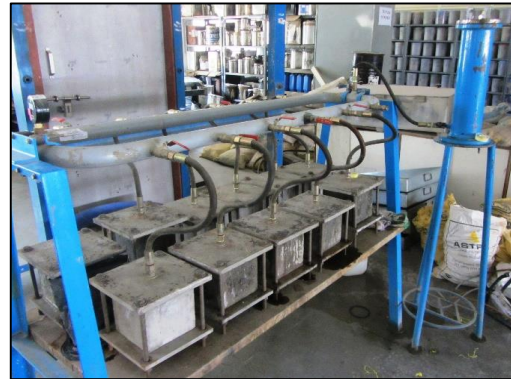
Fig. 6: Permeability test setup
