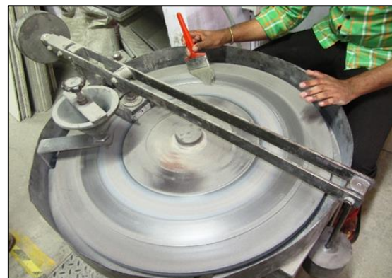
Fig. 10: Abrasion Resistance test setup
