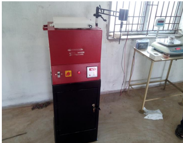
Fig. 1: Stir Casting Setup
