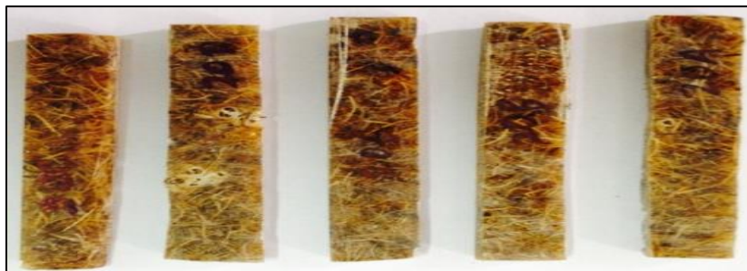
Fig. 7: Specimen prepared for IZOD impact test (A) 10 phr (B) 20 phr (C) 30 phr.
