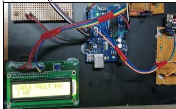
Fig. 11: Cable Fault at 3km
