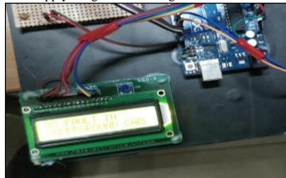
Fig. 10: No Cable Fault Found
